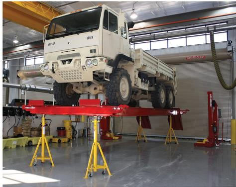
Height adjustment in 25.4mm with 101mm fine-tuning.
