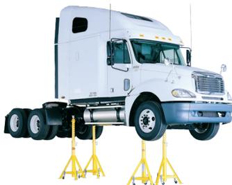
*Always use safety stands when installing or removing heavy components.*
